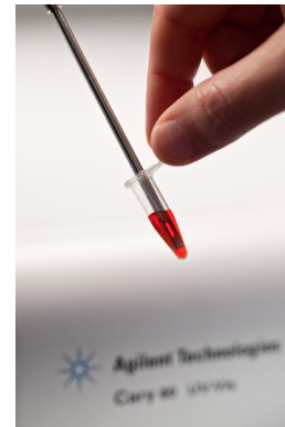
Fiber optic dip probes
