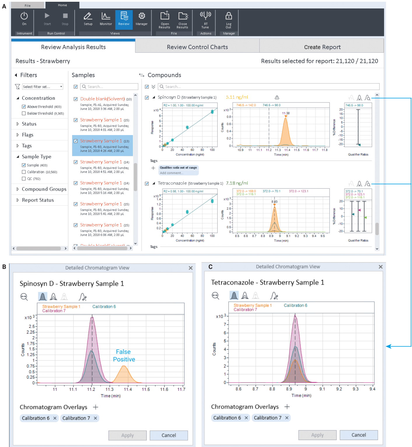
Figure 4. (A) Identified Spinosyn D and Tetraconazol in a nonorganic strawberry sample. (B, C) Overlaid plots of quantifier ion of identified pesticides in nonorganic strawberry and two calibration samples. (B) shows the incorrect RT for the Spinosyn D quantifier ion in nonorganic strawberry compared to two calibration samples (false positive identification). (C) shows the correct RT for standard Tetraconazol in calibration and nonorganic strawberry samples (true identification).
