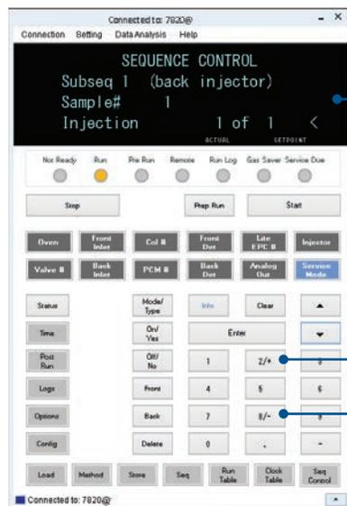
Pressure (or flow) values are digitally displayed and adjusted manually. There are no pressure or flow set points that can be entered or saved to a method.
